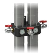
6 By opening the stopcock on the water outlet side, the home supply is put into operation. The water outlet side is marked by a label. In order to remove already existing contaminations from the piping system, the water should flow for approx. 2-3 minutes from each tap in the house after the QUADRO installation has been completed. It is advantageous to clean all the aerators in the house in order to wash out the coarsest dirt.
