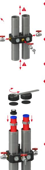
Fasten the wall holder to the wall using suitable fastening material (plugs, screws).
